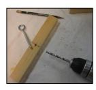
12. Place a nut and washer on a long screw eye and
