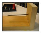
7. On the "inside," shape a hook of approximately 0.5-inch diameter. On the "outside," bend the wire to form a crank with two kinks.
